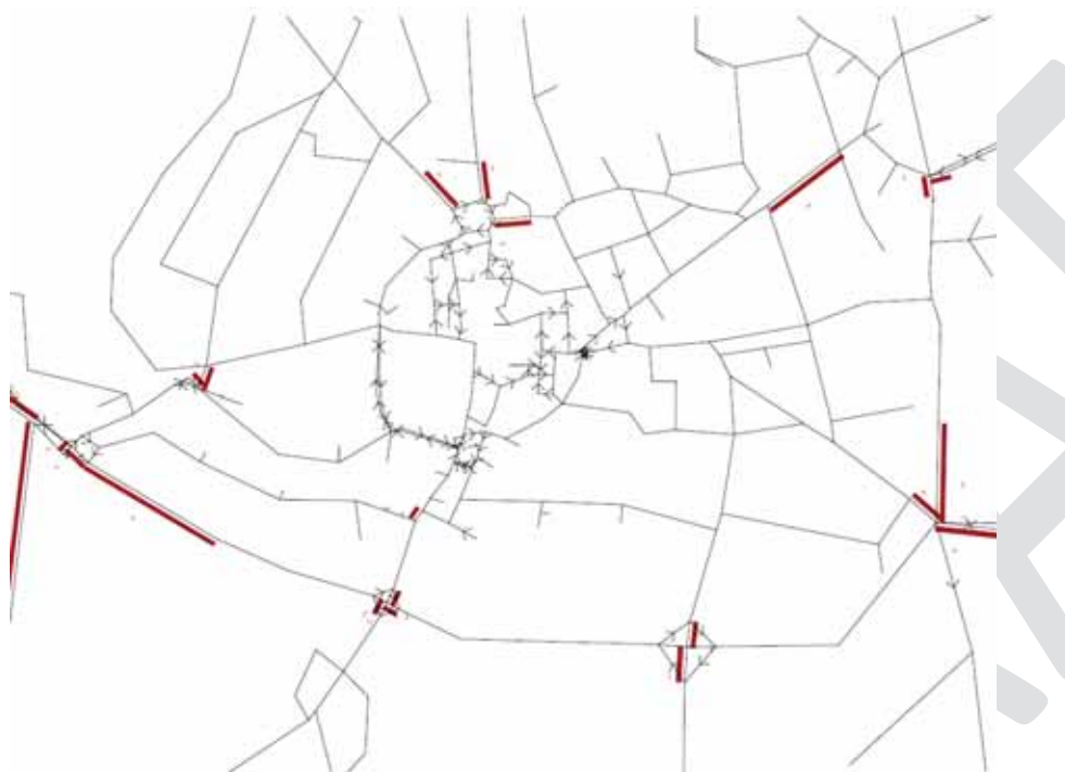
Figure 4.8: Option 5 Link Flow to Capacity Ratio >95% (AM Peak)
