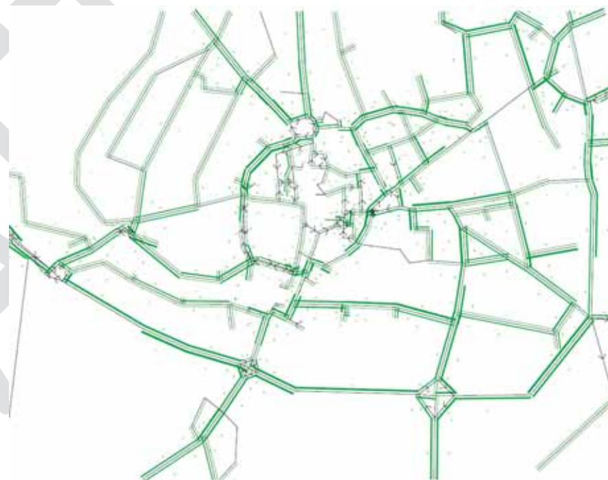
Figure 6.7: Option 6-11 Link Flow to Capacity Ratio <75% (PM Peak)
