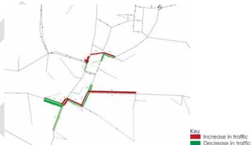
Figure 2.4: PM Base model compared to traffic counts (after calibration)
