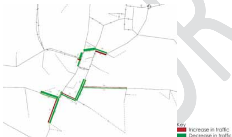
Figure 2.3: AM Base model compared to traffic counts (after calibration)
