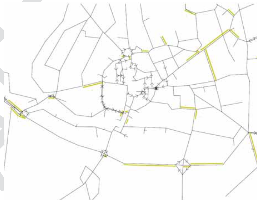
Figure 6.9: Option 6-11 Link Flow to Capacity Ratio >75% and <95% (PM Peak)
