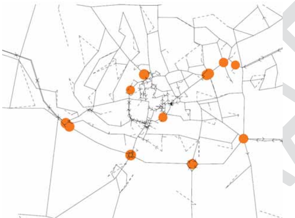
Figure 3.12: 2035 DM - Flow to Capacity Ratio >75% and <95% (AM Peak)
