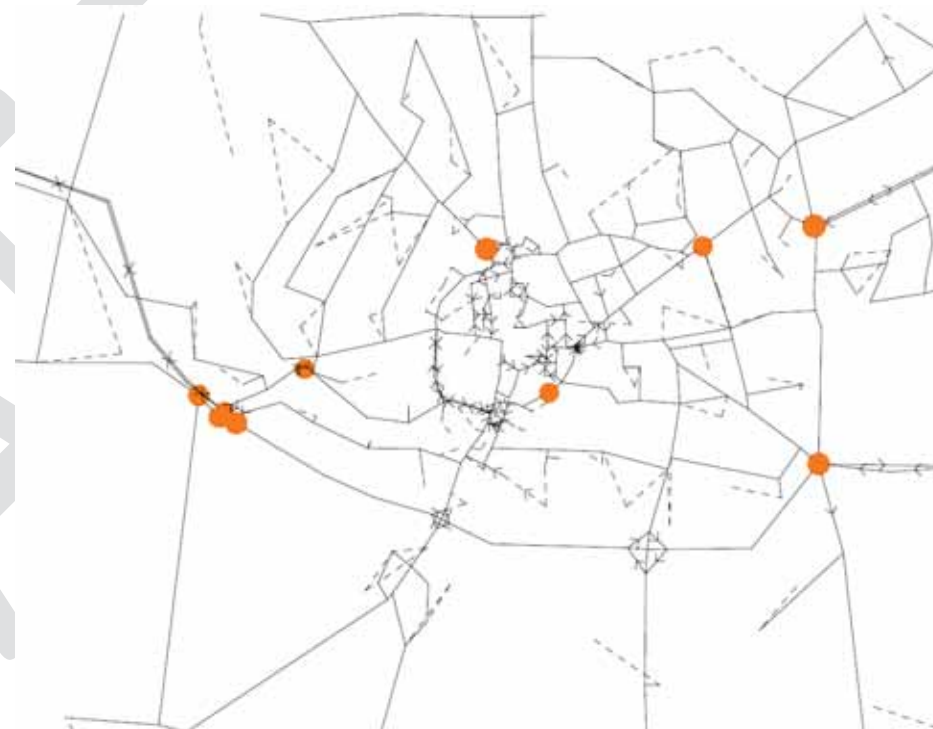
Figure 4.13: Option 5 Flow to Capacity Ratio >75% and <95% (PM Peak)
