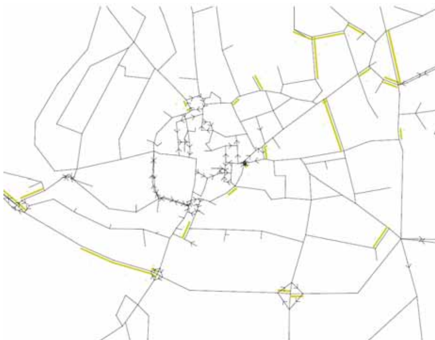
Figure 5.8: Option 10 Link Flow to Capacity Ratio >75% and <95% (AM Peak)
