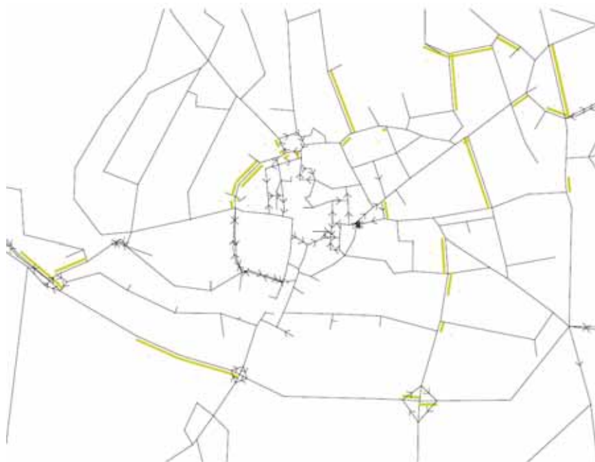
Figure 8.8: Option 9 Link Flow to Capacity Ratio >75% and <95% (AM Peak)
