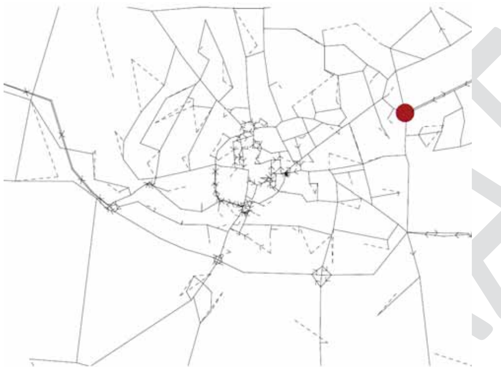
Figure 3.14: 2035 DM - Flow to Capacity Ratio >95% (AM Peak)
