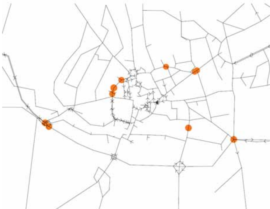
Figure 8.14: Option 9 Flow to Capacity Ratio >75% and <95% (AM Peak)
