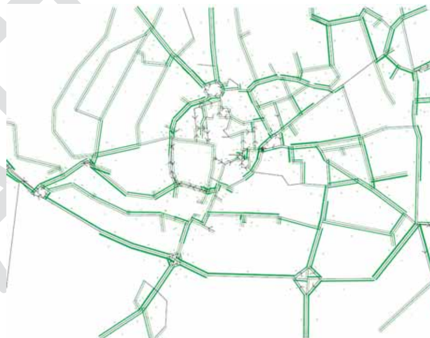
Figure 7.7: Option 8 Link Flow to Capacity Ratio <75% (PM Peak)
