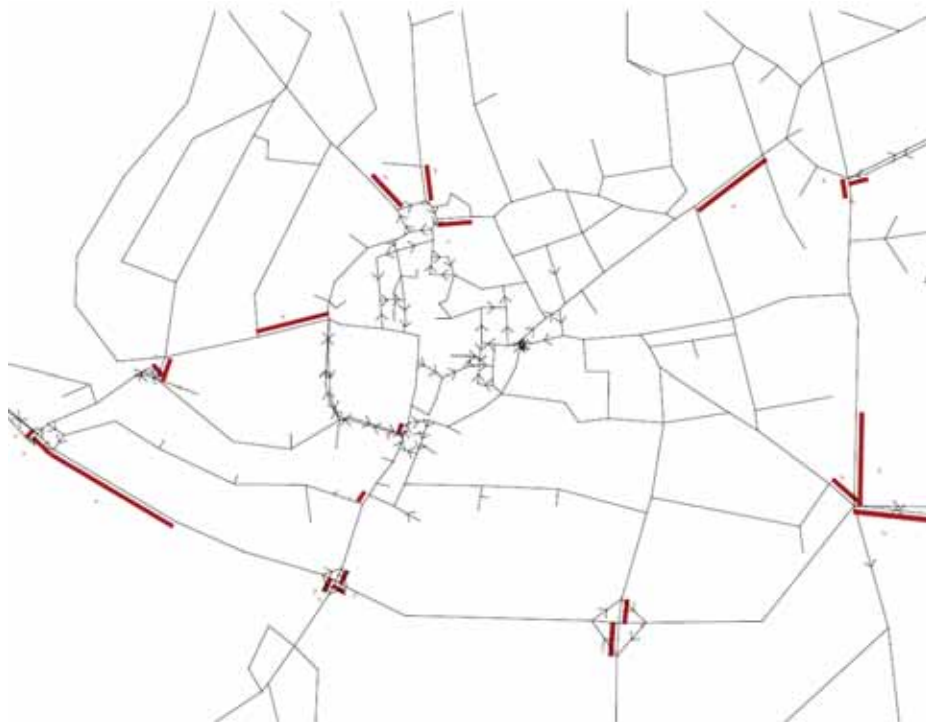
Figure 5.10: Option 10 Link Flow to Capacity Ratio >95% (AM Peak)
