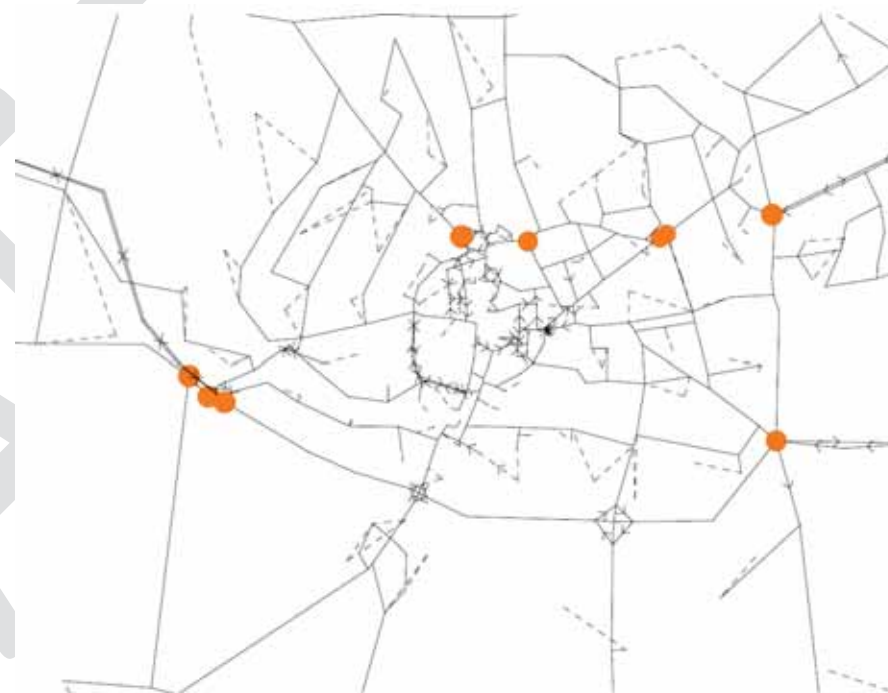
Figure 8.15: Option 9 Flow to Capacity Ratio >75% and <95% (PM Peak)
