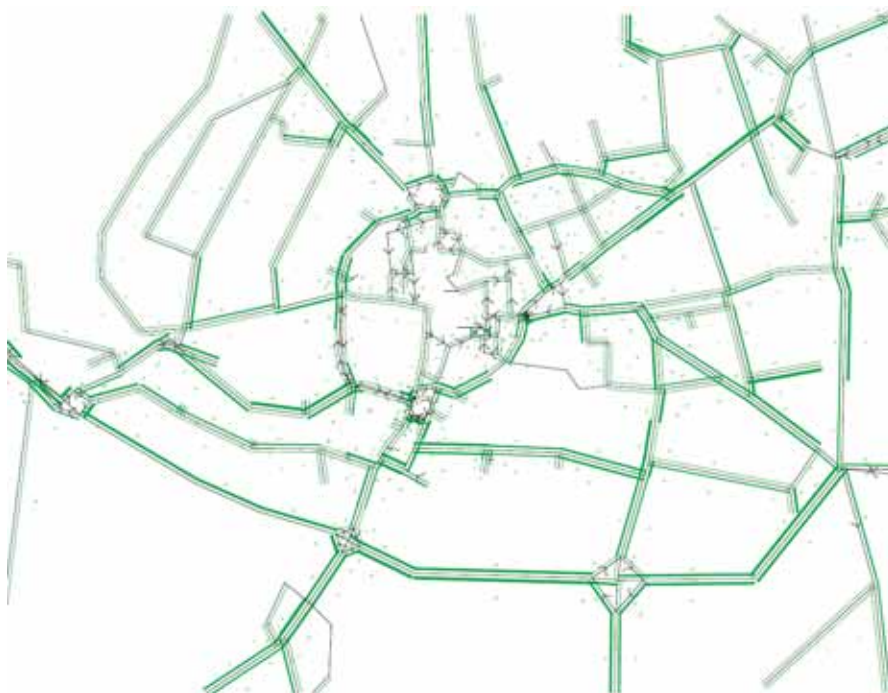
Figure 4.4: Option 5 Link Flow to Capacity Ratio <75% (AM Peak)
