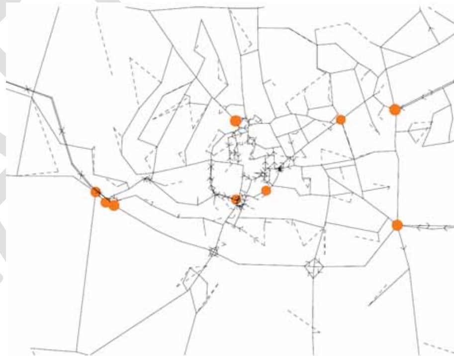
Figure 3.13: 2035 DM - Flow to Capacity Ratio >75% and <95% (PM Peak)
