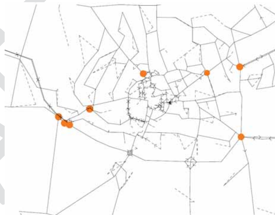
Figure 7.15: Option 8 Flow to Capacity Ratio >75% and <95% (PM Peak)
