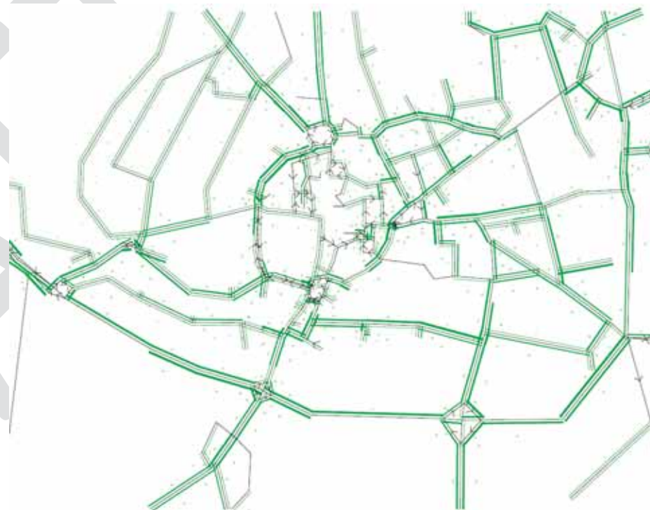
Figure 4.5: Option 5 Link Flow to Capacity Ratio <75% (PM Peak)
