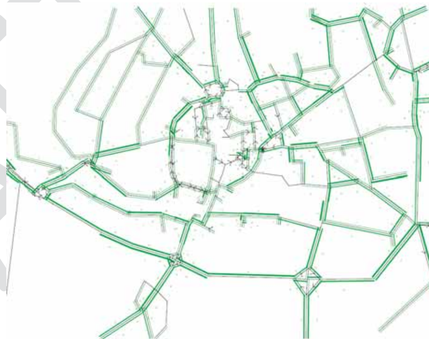
Figure 8.7: Option 9 Link Flow to Capacity Ratio <75% (PM Peak)
