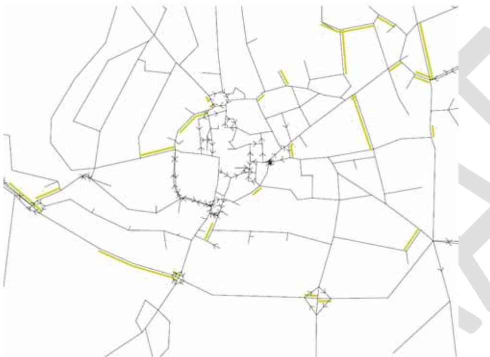
Figure 4.6: Option 5 Link Flow to Capacity Ratio >75% and <95% (AM Peak)
