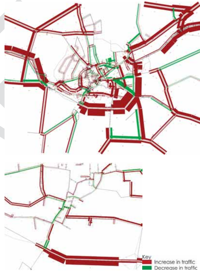
Figure 3.3: 2035DM (with development) vs 2014 Base (PM Peak)
