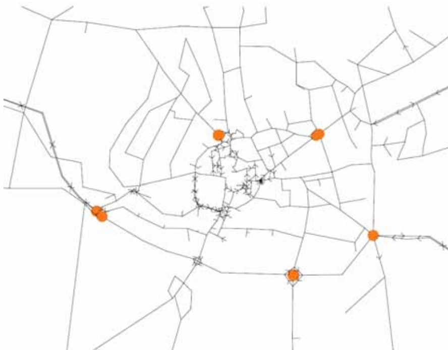
Figure 5.14: Option 10 Flow to Capacity Ratio >75% and <95% (AM Peak)
