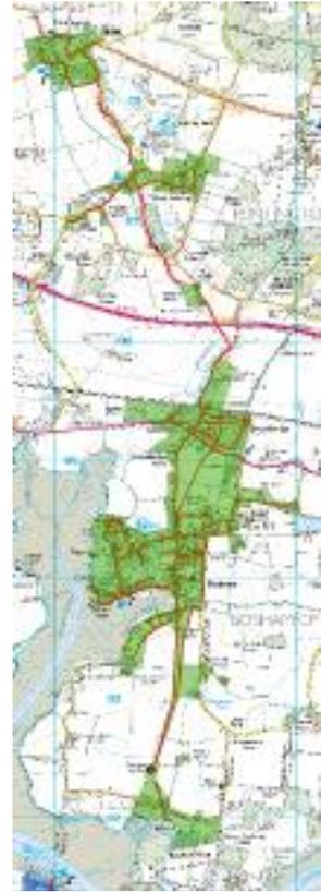
Diagrammatic representation of Bosham known flood locations, fluvial flows and field drainage, including the Colner stream (course of ancient river), Bosham Millstream, the central waterway and the East Ditch systems. The last three are considered by the EA to be 'main rivers' and as such enjoy the benefit of EA management. The diagram overlays the 2014 SHLAA map
