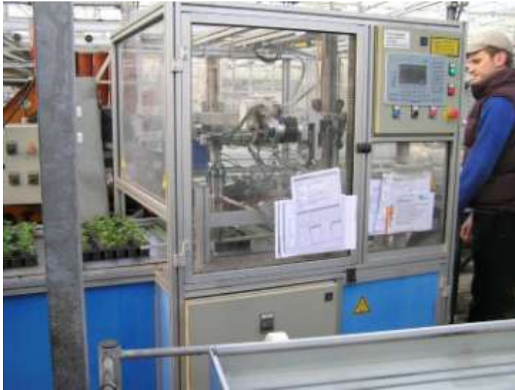
Figure 34 Robot Transplanter for Containerised Plants
