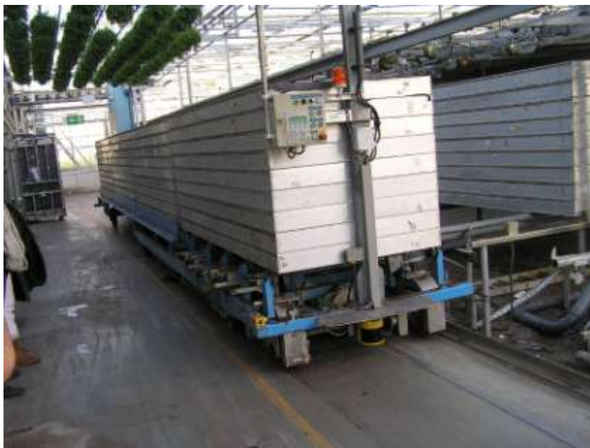
Figure 31: Automated Loading of Robotic Transport System
