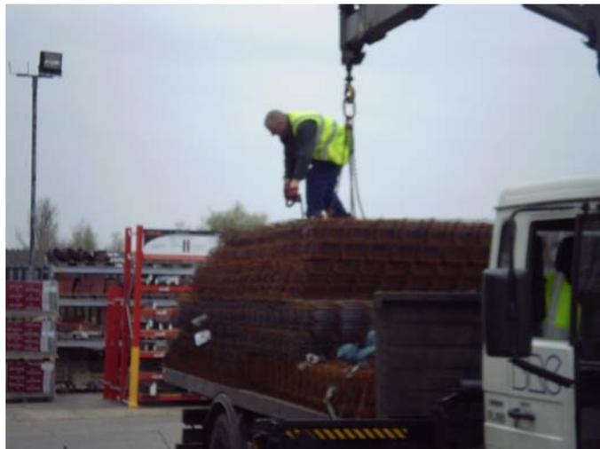
2. Some of the articulated trailer units fitted out in the UK had inadequate access. The only ladder was a pull-out one at the rear with no hand holds above the flat bed. This issue was raised with the HSE.
